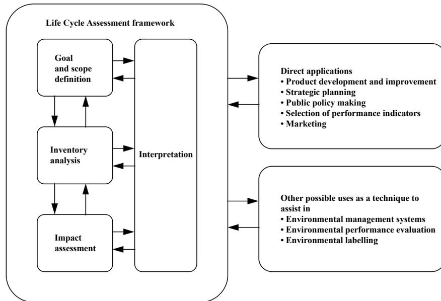
**Figure 1. The LCA methodology and framework** (Source: ISO 14040:1997)
