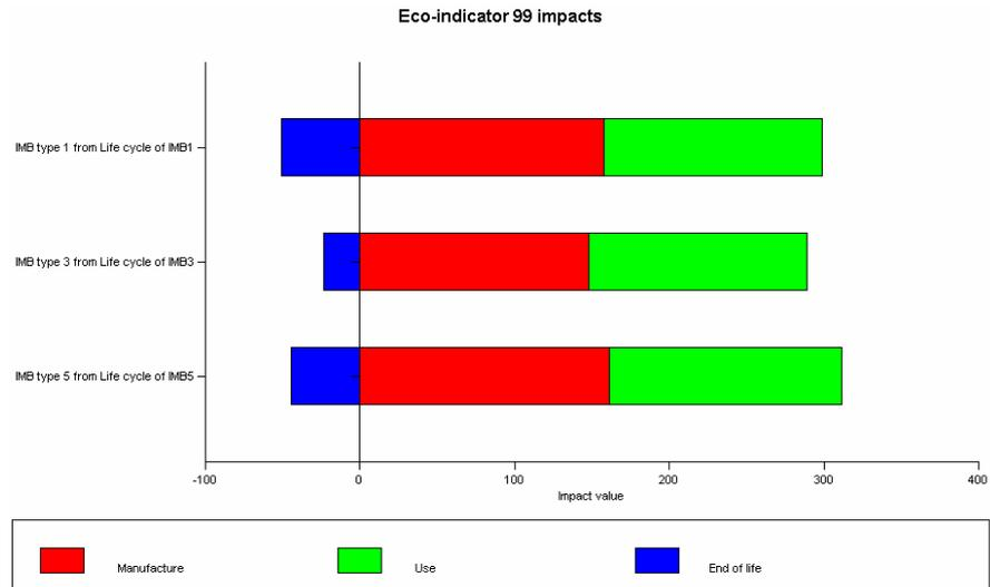
**Figure 6: Life cycle impact of IMB type 1, 3 and 5 using the Eco indicator 99 weighting method.**
