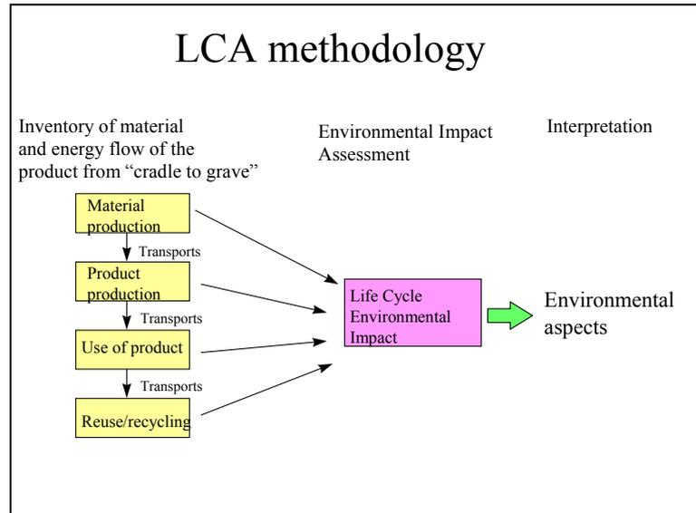
**Figure 2. Basic principle of the LCA methodology.**
